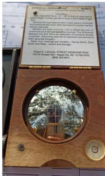
Figura 7. *Emispherical densiometer*
